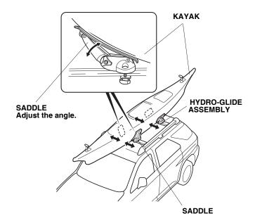
Slide the kayak forward or backward until it's level with the roof. If necessary, loosen the knob on each saddle and adjust the saddle angle to fit snugly against the kayak. Tighten each knob securely. 6. Route each strap with buckle through the buckle cover with the ribbed side facing up.
