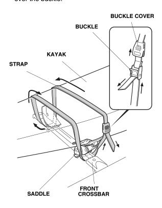
Route the strap under the rear crossbar, and around the kayak as shown. Slide the buckle cover away from the buckle, route the strap through the buckle, and tighten the strap. Slide the buckle cover back over the buckle.
