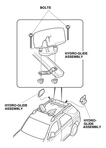
3. Rest the front of the kayak on the hydro-glide assemblies. Standing behind or alongside the kayak, lift up the rear of the kayak and push it forward onto the hydro-glide assemblies and saddles. Make sure the kayak reaches the front saddles before you lower it
